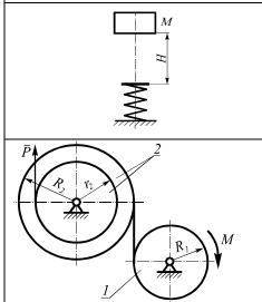
24. The load M of mass m = 0.5 kg falls without initial velocity from the height H = 1.2 m and reaches the spring with the stiffness coefficient c = 196 N/m. Determine the value of maximal spring compression h.
