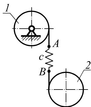
Homogeneous disks 1 and 2 have the same mass  $m$  and radii  $r$ . The discs are in the vertical plane. The discs are linked by a vertical inextensible thread with an elastic part  $AB$  having the coefficient of elasticity  $c$ . At initial moment the system rested and the spring  $AB$  was unstretched.
