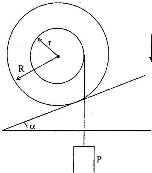
A stepped block whose radii are  $r$  and  $R$ , and the force of gravity is  $G$ , is located on an unsmooth inclined plane. A thread is wound on the inner step of the block; a load is suspended to the end of the thread. The coefficient of friction of adhesion between the block and the plane is  $f$ .
