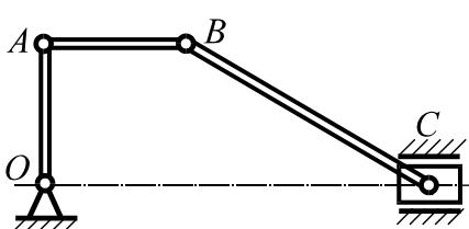
The presented mechanism includes rods  $OA$  and  $AB$  of the same length and a rod  $BC$ , which is twice longer. Velocities of points  $A$  and  $C$  are equal by modulo, constant and at the demonstrated time moment they are directed in the opposite sides.
