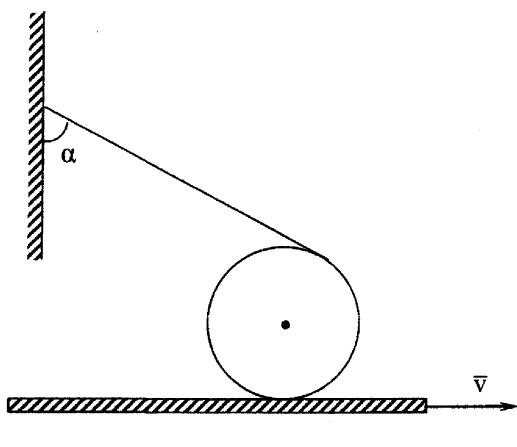
A cylinder of radius  $r$  is wrapped by a thread. The second end of the thread is connected to a vertical wall. The cylinder is placed on a horizontal desk moving translationally along the horizontal direction with a constant Velocity  $v$ . There is no slipping between the cylinder and the desk.
