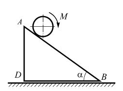
The triangle prism of mass 2m is placed on the smooth horizontal plane. An angle at a base of the prism is  $\alpha$ . On the edge AB of the prism a solid homogeneous cylinder of mass m and radius r rolls under the action of moment M. The friction coefficient between the cylinder and the prism is f.
