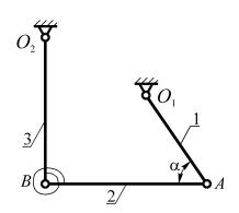
In a rod system located vertically, rods 1, 2, and 3 have lengths  $l_1$ ,  $l_2$ ,  $l_3$  and weights  $P_1$ ,  $P_2$ , and  $P_3$ , respectively. Rods 2 and 3 are connected by a spiral spring, which ensures the balance of the system in the position shown in the figure, in which the rod AB is horizontal.
