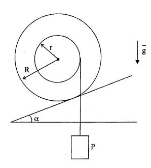
A stepped block whose radii are r and R, and the force of gravity is G, is located on an unsmooth inclined plane. A thread is wound on the inner step of the block; a load is suspended to the end of the thread. The coefficient of friction of adhesion between the block and the plane is f.
