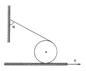
A cylinder of radius r is wrapped by a thread. The second end of the thread is connected to a vertical wall. The cylinder is placed on a horizontal desk moving translationally along the horizontal direction with a constant Velocity v. There is no slipping between the cylinder and the desk.
