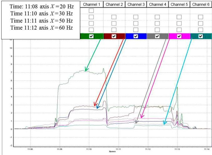
Figure 2 – The frequency-time dependence for the  $X$  axis for the oscillation amplitude equal to 16 mm for the case of RMS base
