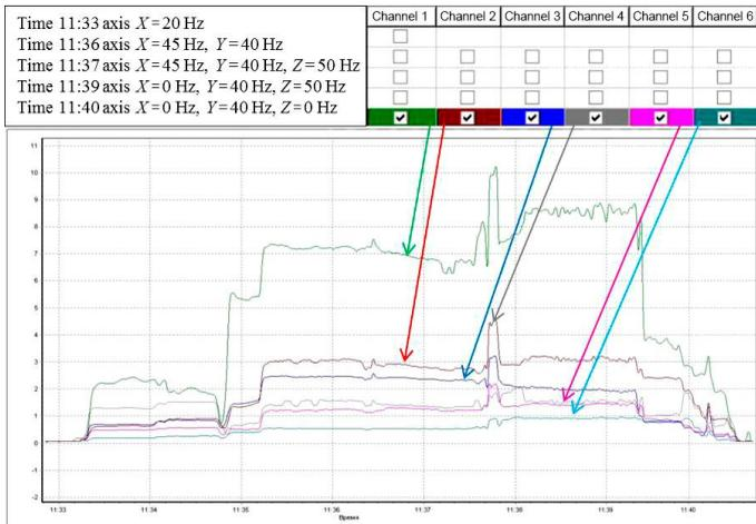
Figure 5 – The frequency-time dependence for the X, Y, Z axes for the oscillation amplitude equal to 16 mm for the case of two RMS in the layout base
