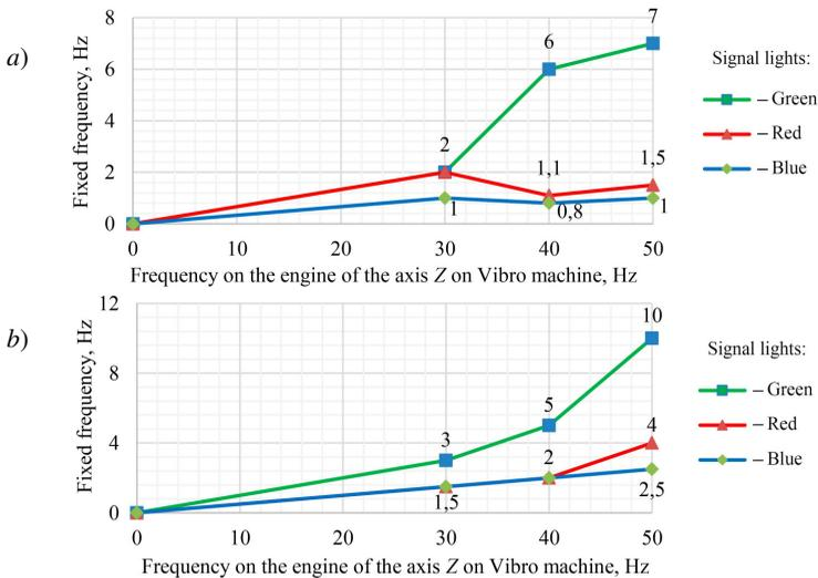
Figure 8 – Sensors' vibrations frequency in Z direction for the case of using RMS with rubber hardness equal to 50 (a), 60 (b)
