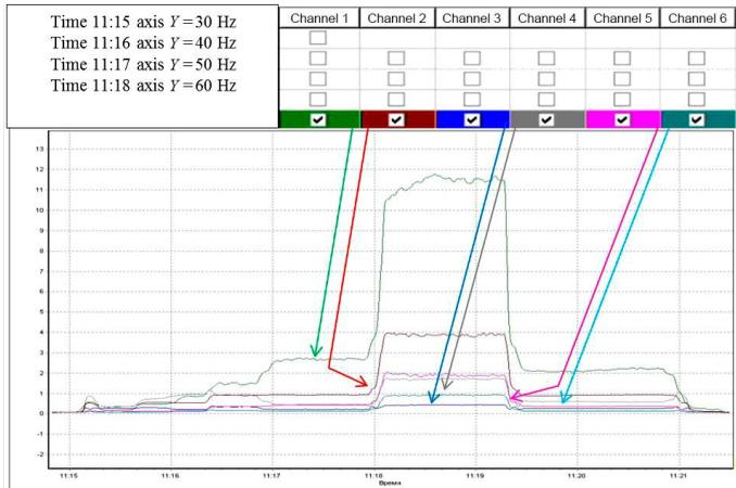
Figure 3 – The frequency-time dependence for the  $Y$  axis for the oscillation amplitude equal to 16 mm for the case of RMS base
