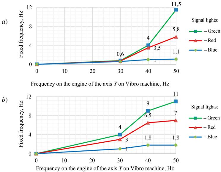
Figure 7 – Sensors' vibrations frequency in Y direction for the case of using RMS with rubber hardness equal to 50 (a), 60 (b)
