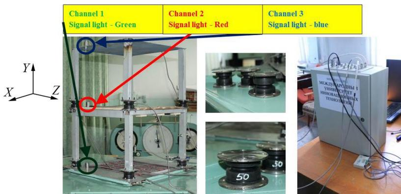
Figure 1 – Layout of the monolithic building, rubber metal supports and STD 2060.1
