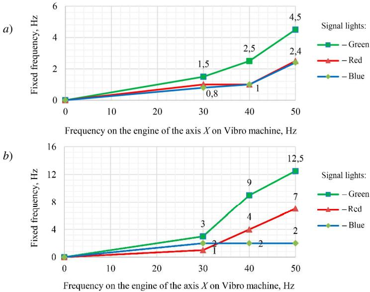
Figure 6 – Sensors' vibrations frequency in X direction for the case of using RMS with rubber hardness equal to 50 (a), 60 (b)
