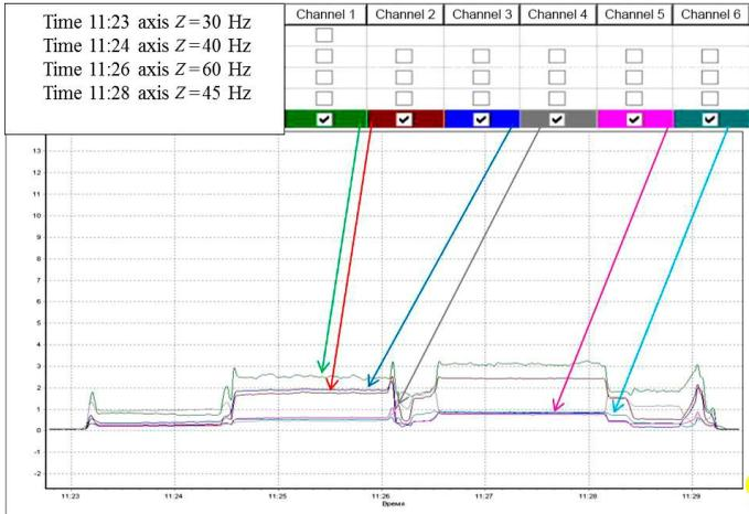
Figure 4 – The frequency-time dependence for the Z axis for the oscillation amplitude equal to 16 mm for the case of RMS base
