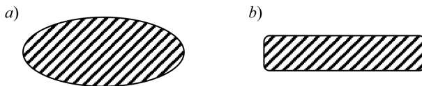
Figure 4 – Cross-section of the ring in the form of a – an ellipse or oval; b – a rectangle
